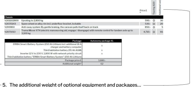
... increases the actual mass of the vehicle (= mass in running order plus selected optional equipment) and reduces the payload. The specified value shows the additional weight compared to the standard equipment of the respective layout. The total weight of the selected packages and optional equipment must not exceed the mass for optional equipment specified by the manufacturer.
